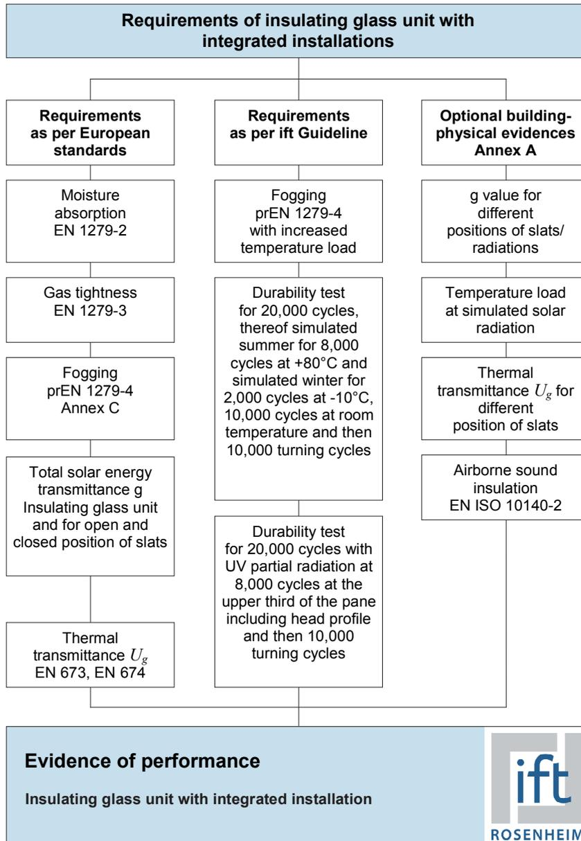
Image 1 Flow chart evidence of fitness for use for IGU with integrated installations
