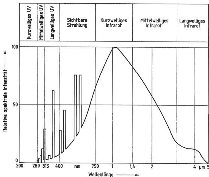
**Image 3** Spectrum of a UV radiation source, e.g. an OSRAM lamp
