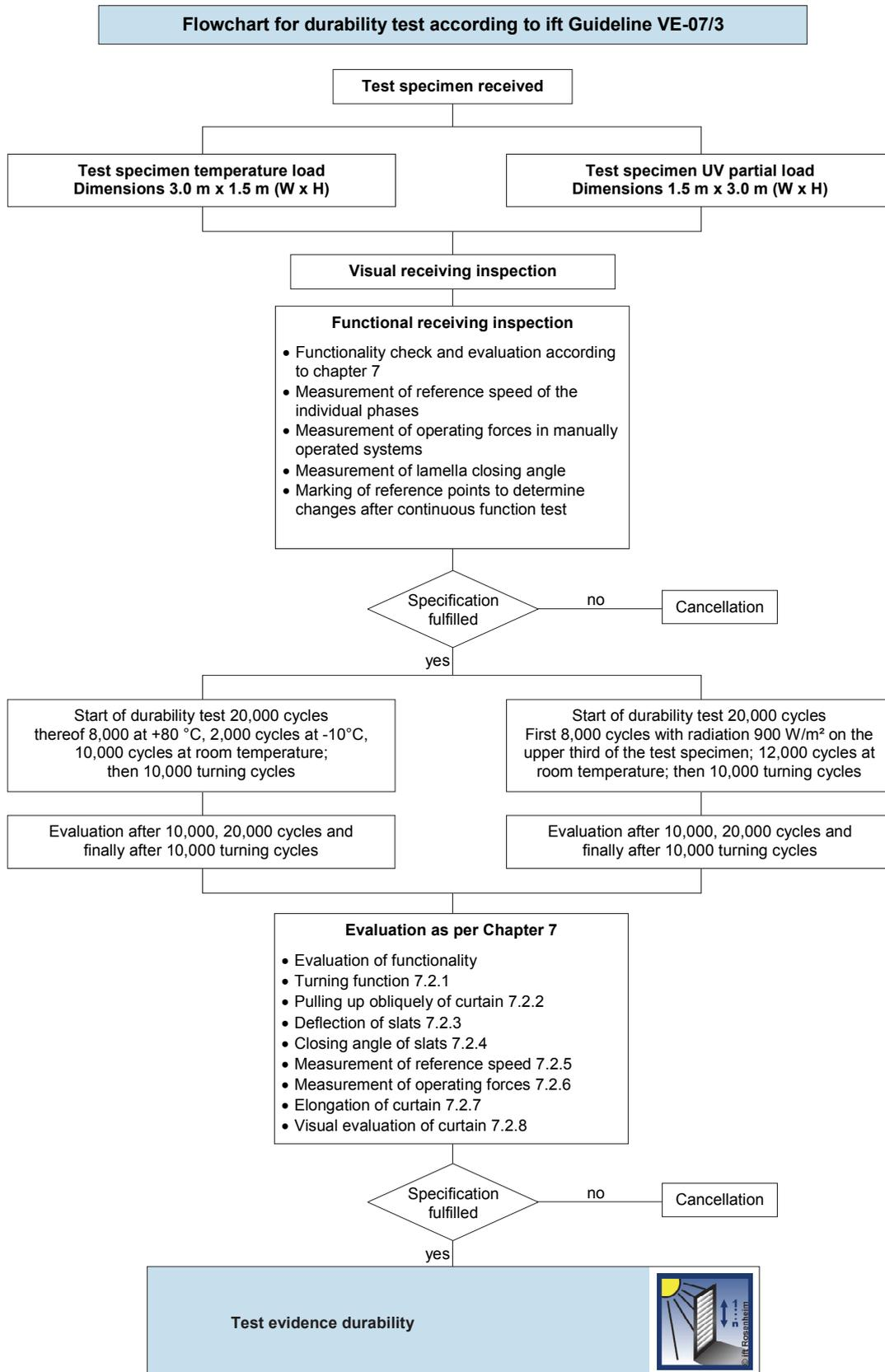
**Image 2** Flow chart of durability test
