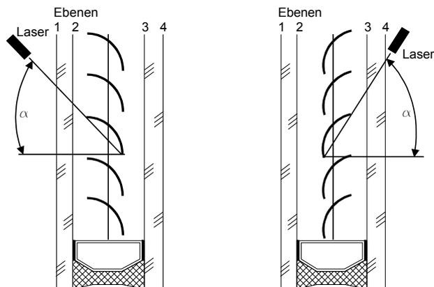
**Image 7** Measurement of the slat angle
