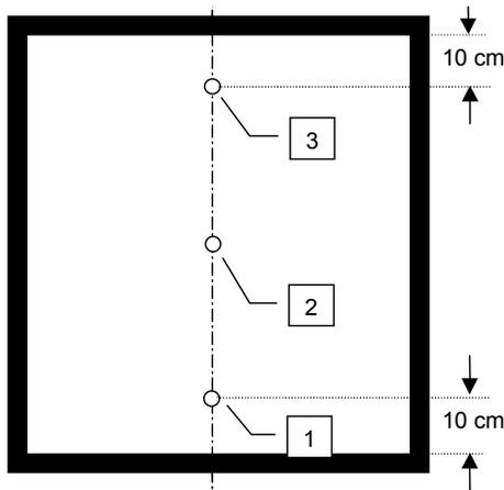
Image A 1 Position of thermocouples
